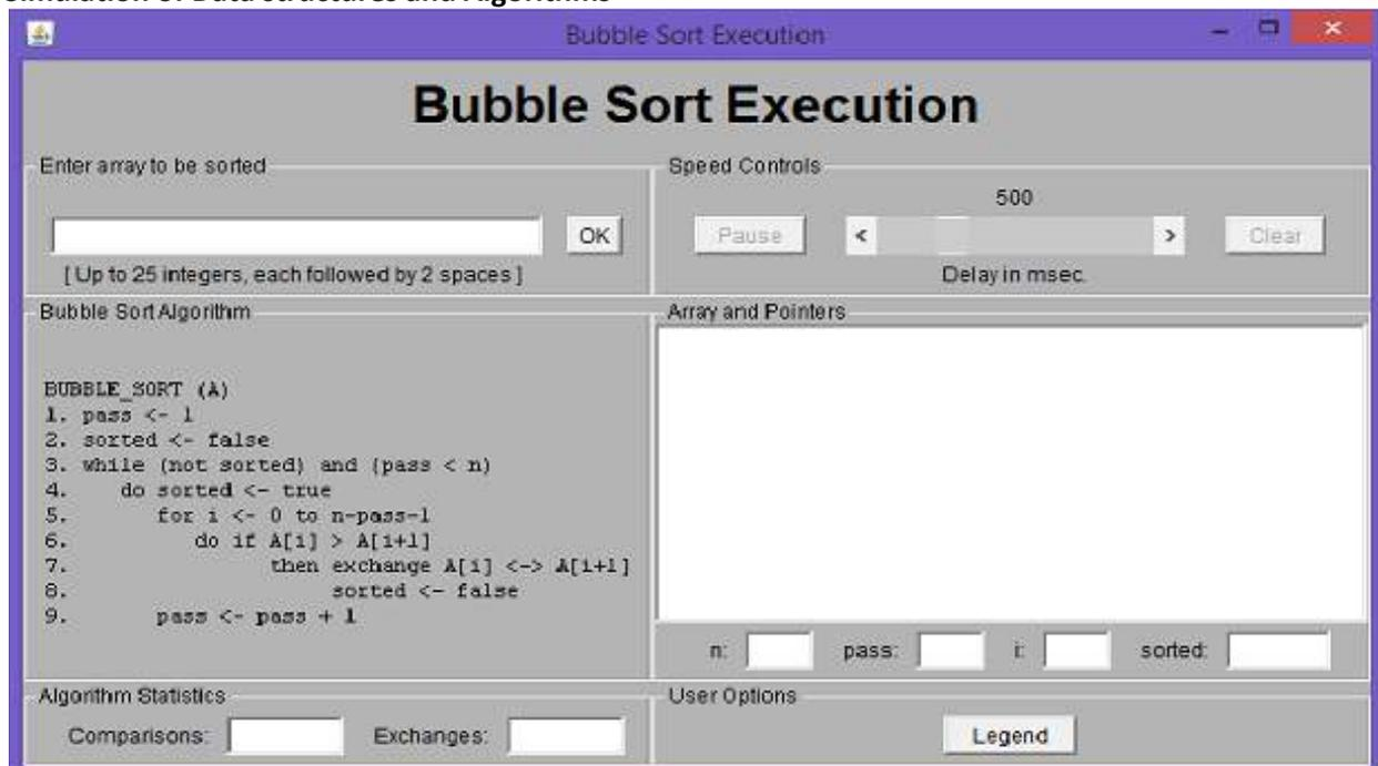
Figure 1: Bubble sort-This contain the text field for input values. The fields in comparisons and Exchanges gives the number of comparison and exchanges. it highlight the current code which is executing.
