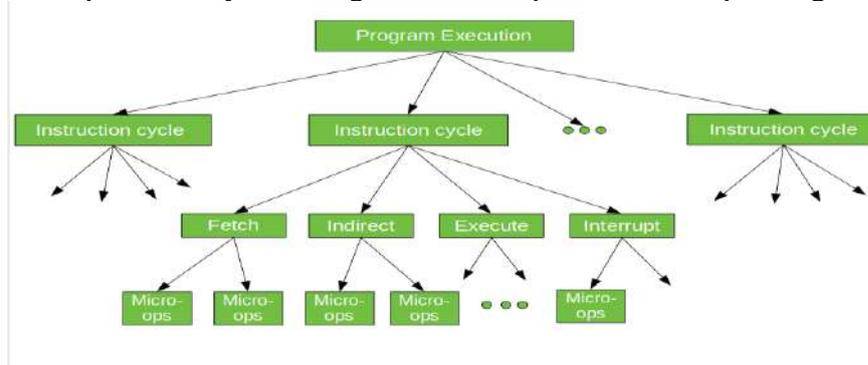
**Summary:** Execution of a program consists of sequential execution of instructions. Each instruction is executed during an instruction cycle made up of shorter sub-cycles(example – fetch, indirect, execute, interrupt). The performance of each sub-cycle involves one or more shorter operations, that is, *micro-operations*.
