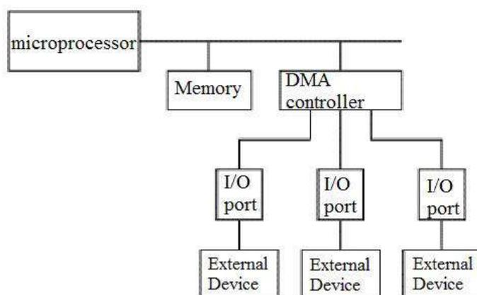
Typical Block Diagram of DMA Controller
